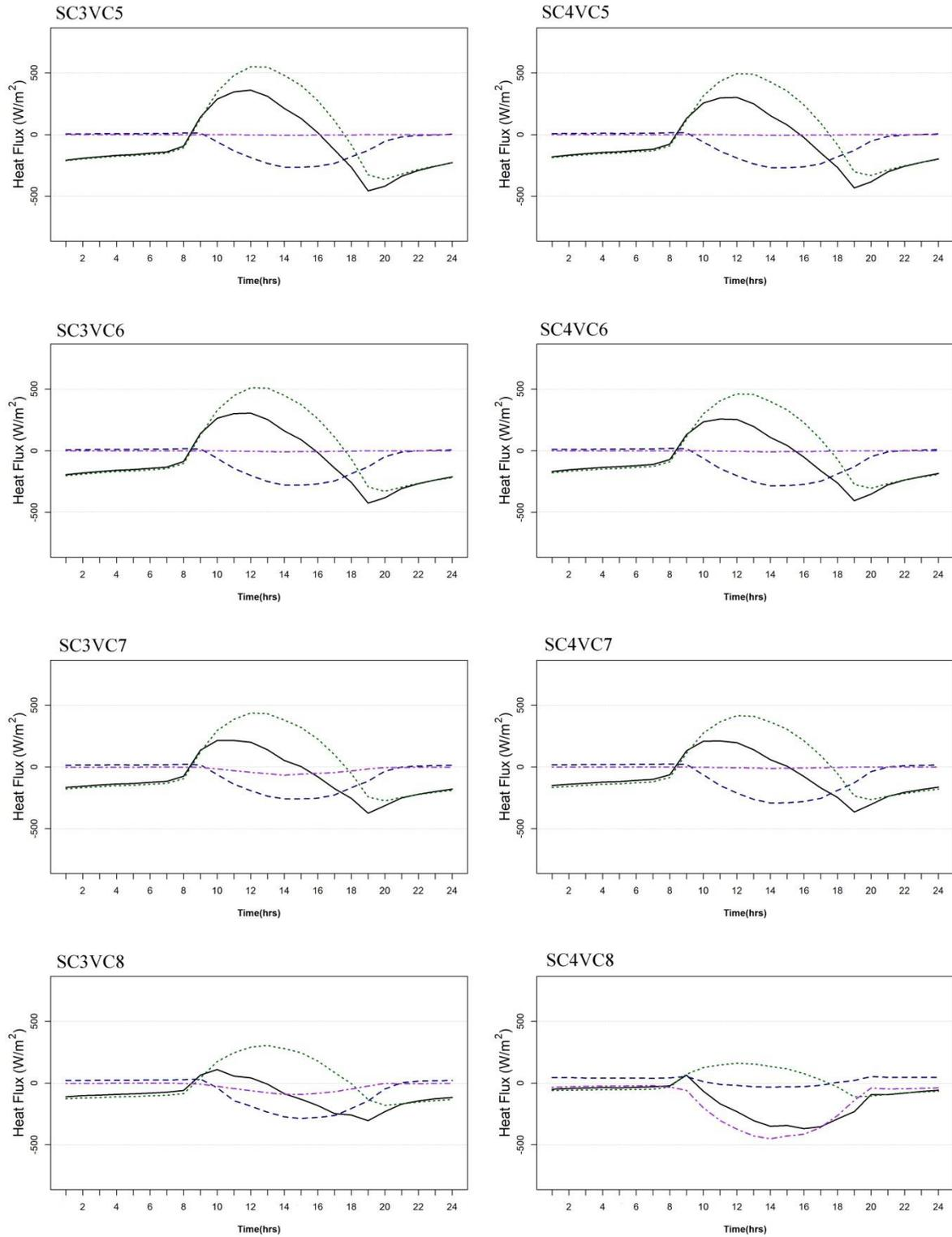
**Figure 5:** Diurnal profiles for net radiation (black solid line), heat storage (green dotted line), sensible heat flux (blue dash line) and latent heat flux (purple dot-dash line) for the different semi-intensive green roof scenarios
