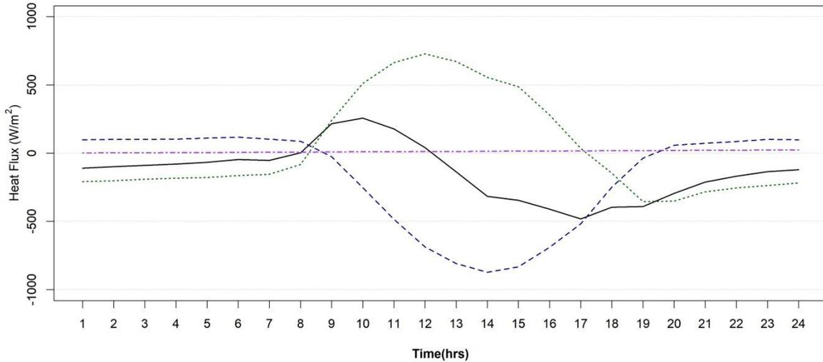
**Figure 6:** Diurnal profile of conventional roof's heat fluxes for net radiation (black solid line), heat storage (green dotted line), sensible heat (dash blue line) and latent heat (dot dash purple line)
