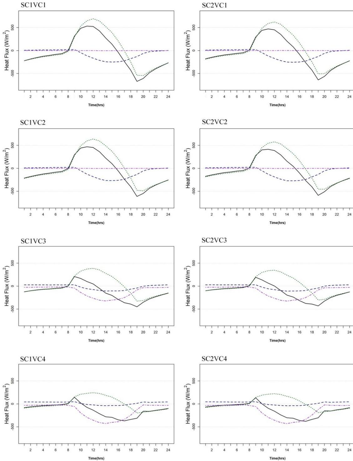
**Figure 4:** Diurnal profiles for net radiation (black solid line), heat storage (green dotted line), sensible heat flux (blue dash line) and latent heat flux (purple dot-dash line) for the different extensive green roof scenarios
