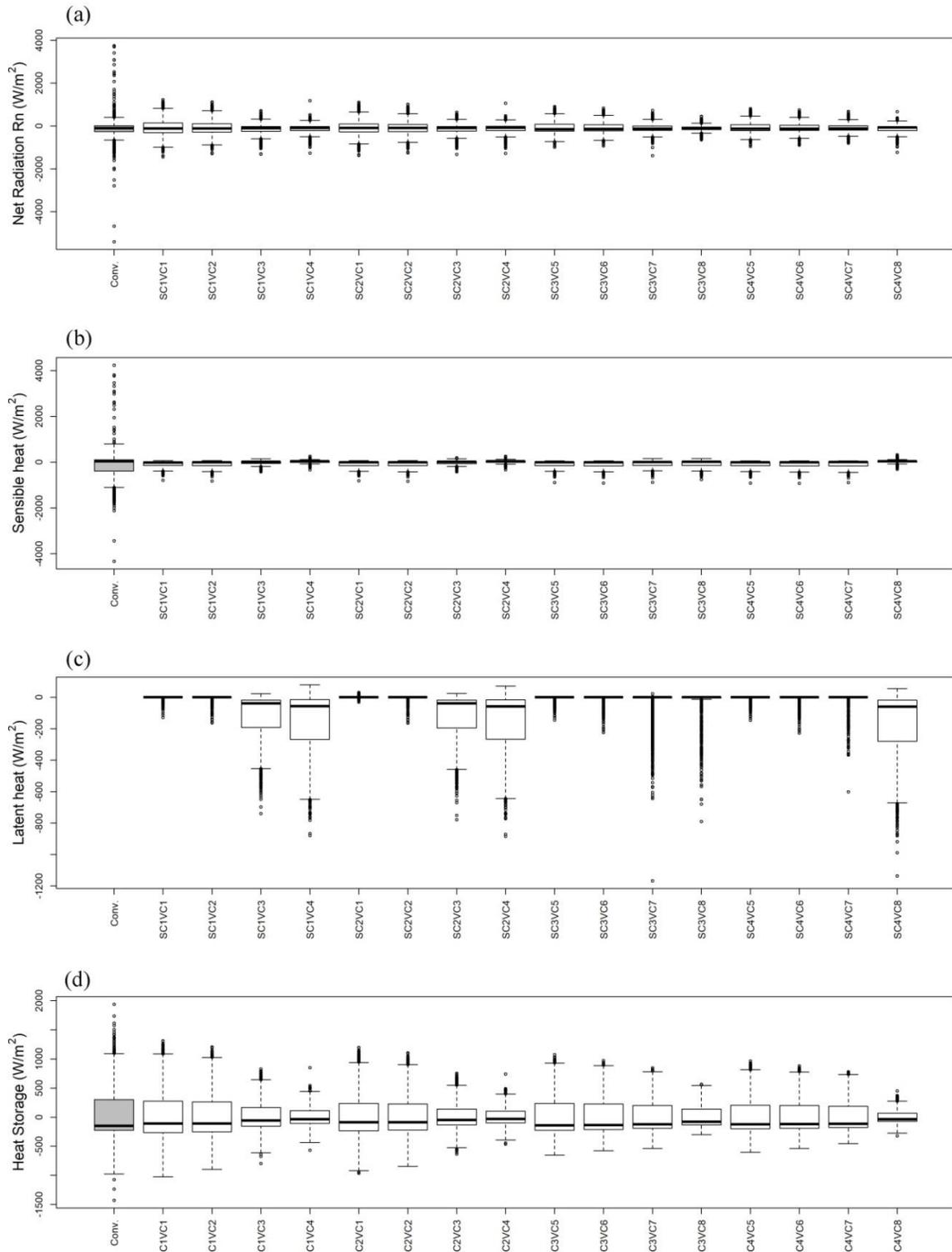
Figure 3: Boxplots of (a) Net radiation, (b) Sensible heat, (c) Latent heat and (d) Heat storage for the conventional roof (grey box) and the different green roof scenarios using hourly measurements
