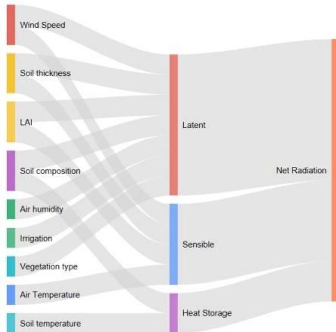
Figure 2: List of parameters affecting the investigated heat fluxes
