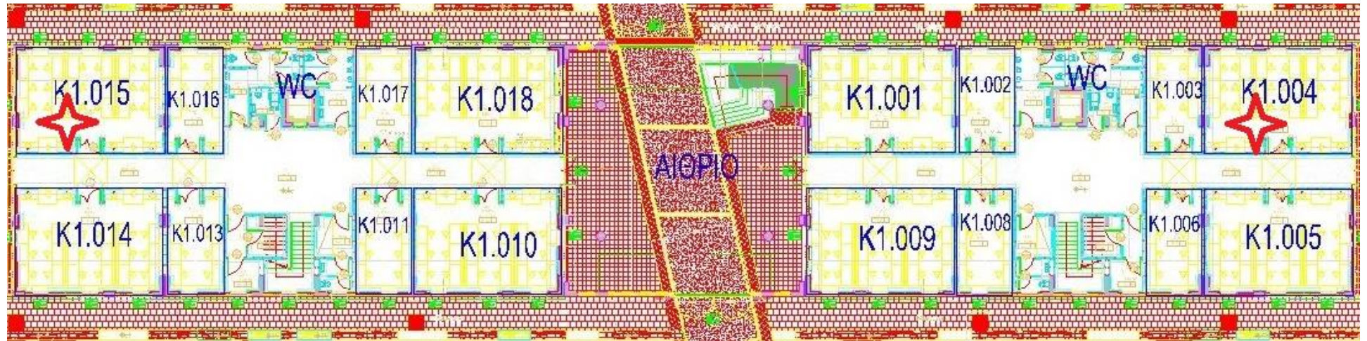
Figure 36: Position of the sensors and actuators on the ground floor of K1 building
