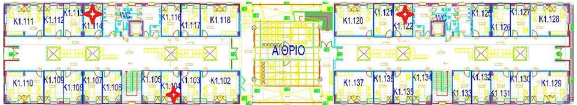
Figure 37: Position of the sensors and actuators on the 1st floor of K1 building
